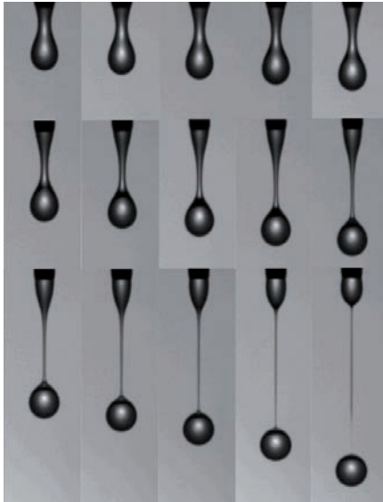
Sequence of images depicting the formation of PDMS silicone oil droplets taken with GMF's high-speed camera.
